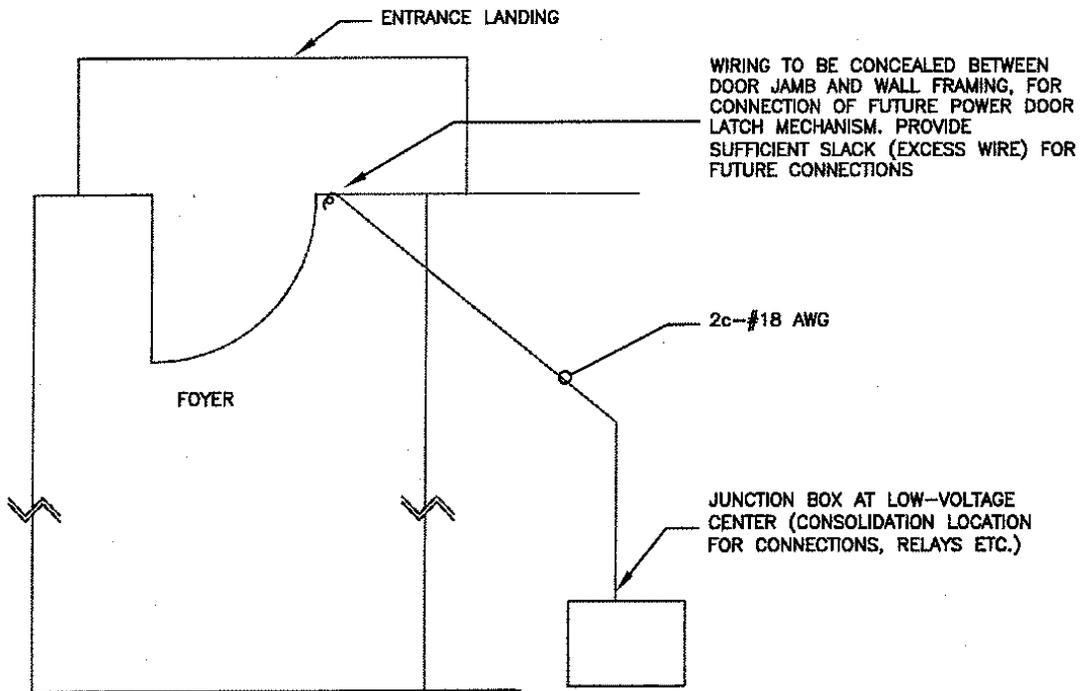
DIAGRAM A.14.6 – ELECTRIC DOOR LOCK RELEASE MECHANISM
