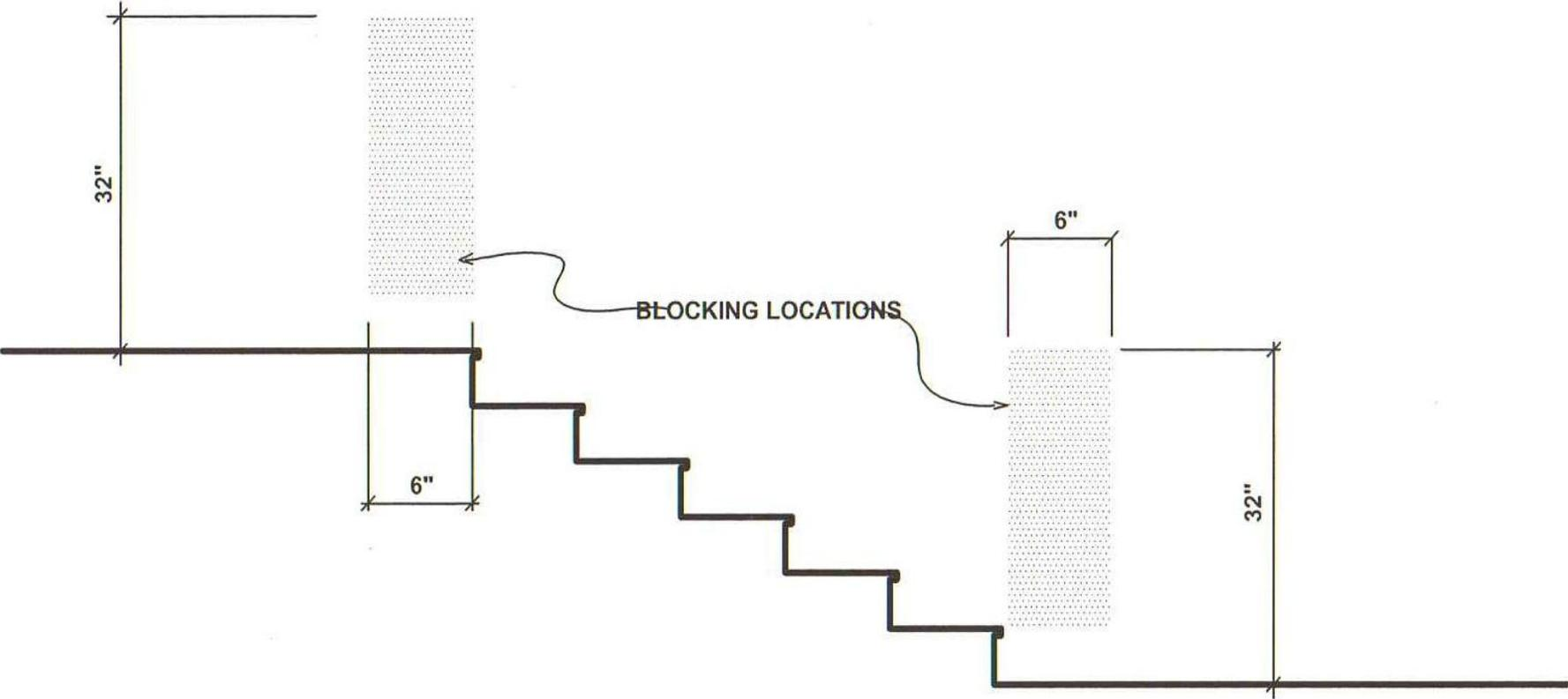
IDEAL HORIZONTAL POSITION OF BLOCKING WILL VARY WITH STAIR AND RAILING DESIGN
